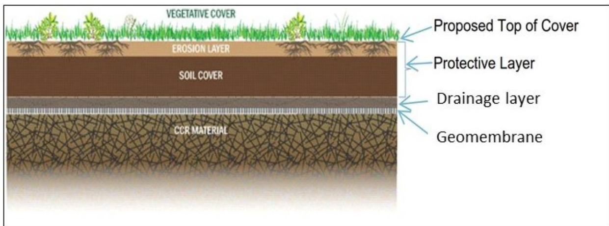
Figure 1: Proposed Alternative Final Cover System
